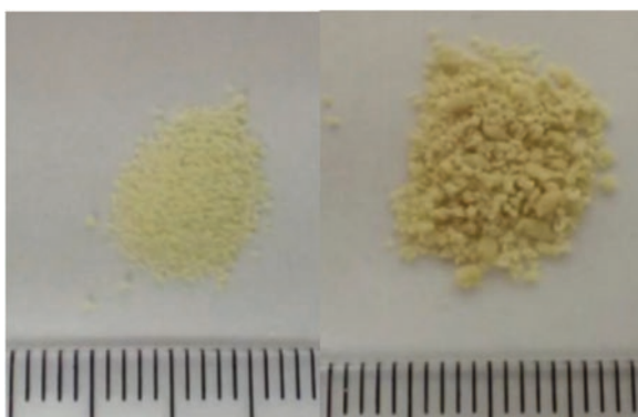
Fig. 3.4 Granulation of powder is performed to improve powder flow in tablet manufacturing. An exemplary powder is shown before (left) and after (right) granulation. Images provided courtesy of S.V. Jermain, University of Texas at Austin
