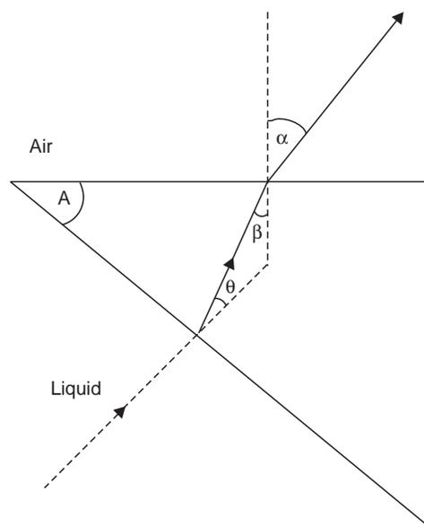
Figure 18.4. Abbe' Refractometer : Optical Path
