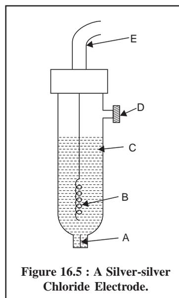
**Figure 16.5 : A Silver-silver Chloride Electrode.**
