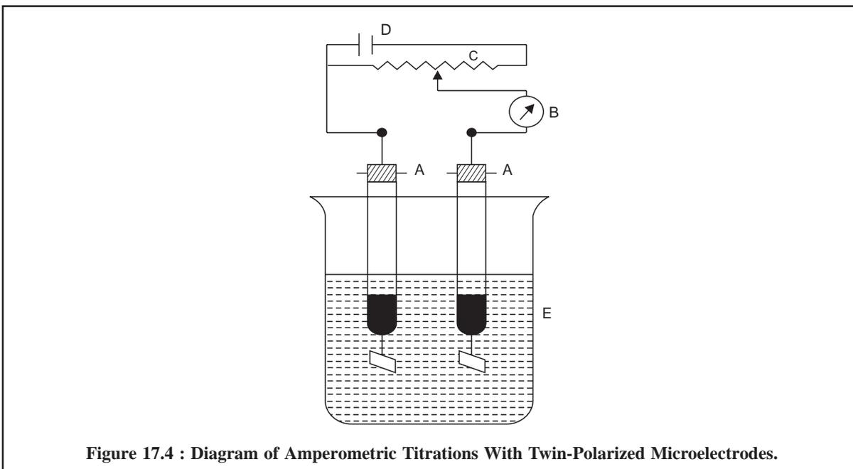
**Figure 17.4 : Diagram of Amperometric Titrations With Twin-Polarized Microelectrodes.**
