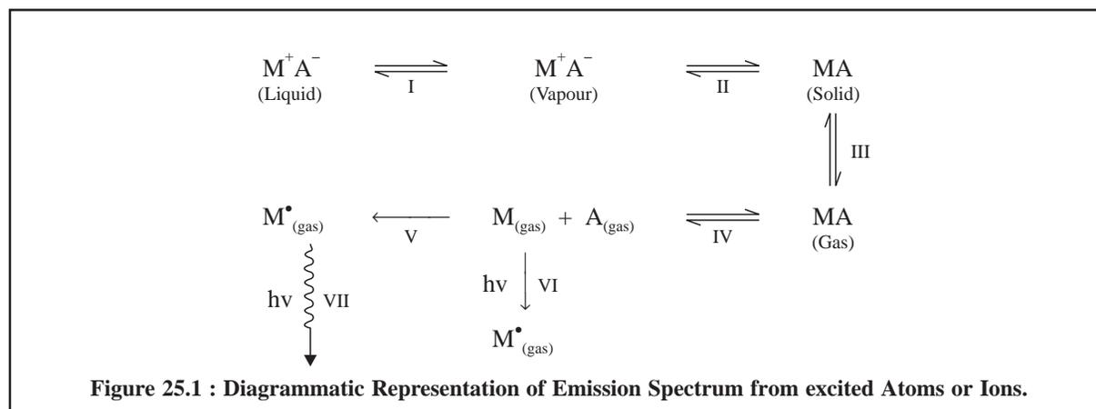
Figure 25.1 : Diagrammatic Representation of Emission Spectrum from excited Atoms or Ions.
