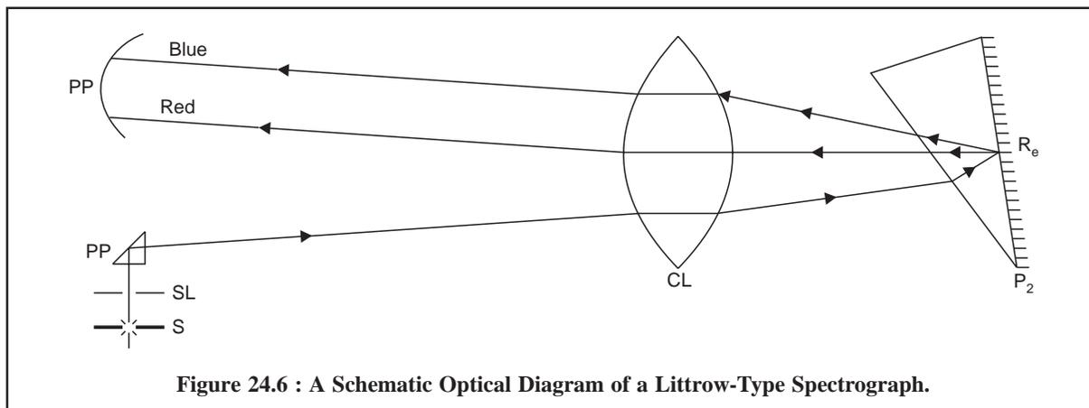
**Figure 24.6 : A Schematic Optical Diagram of a Littrow-Type Spectrograph.**
