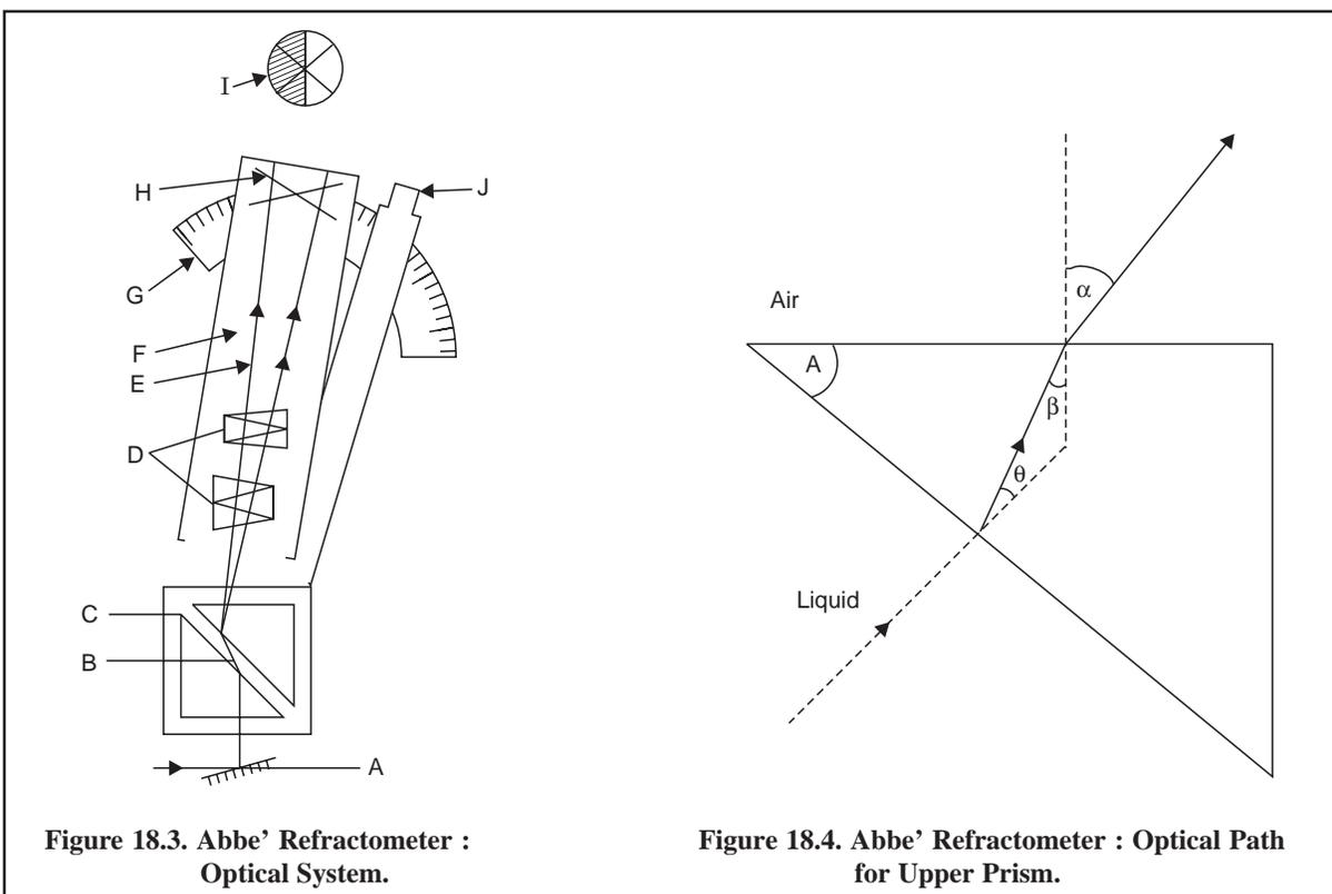
Figure 18.3. Abbe' Refractometer :
