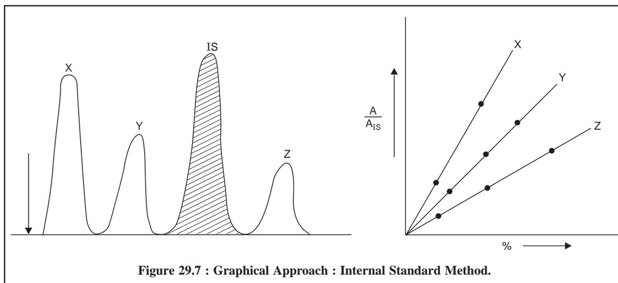
**Figure 29.7 : Graphical Approach : Internal Standard Method.**
