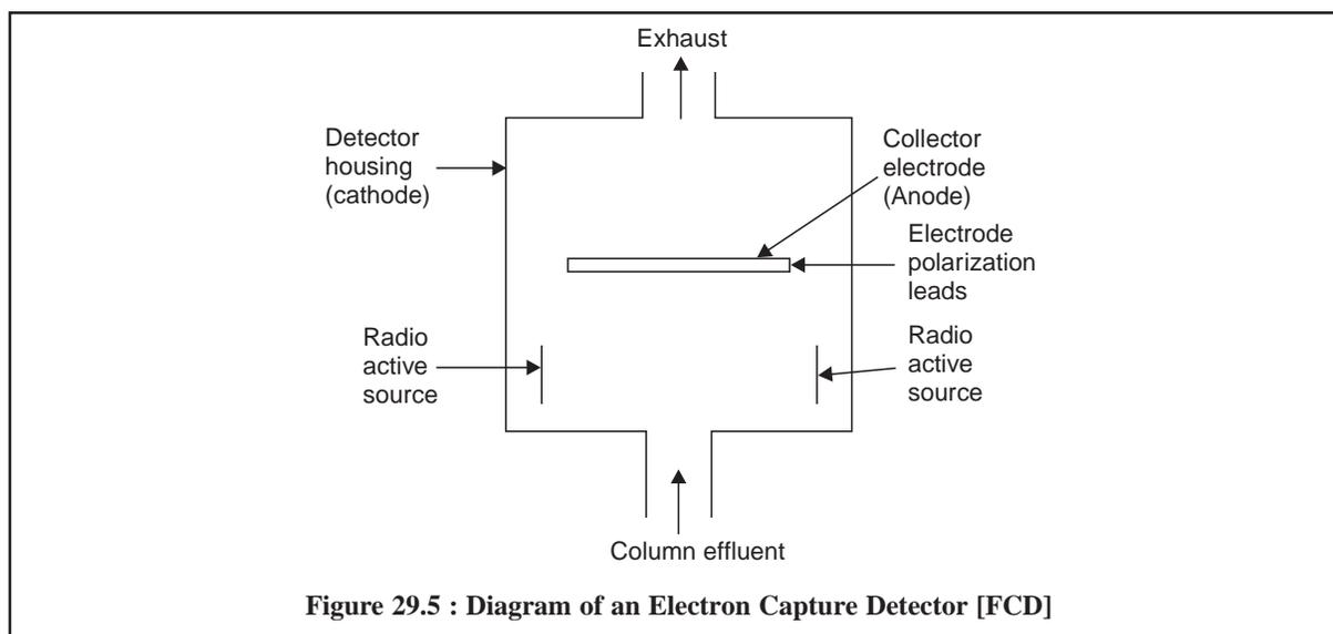
Figure 29.5 : Diagram of an Electron Capture Detector [FCD]
