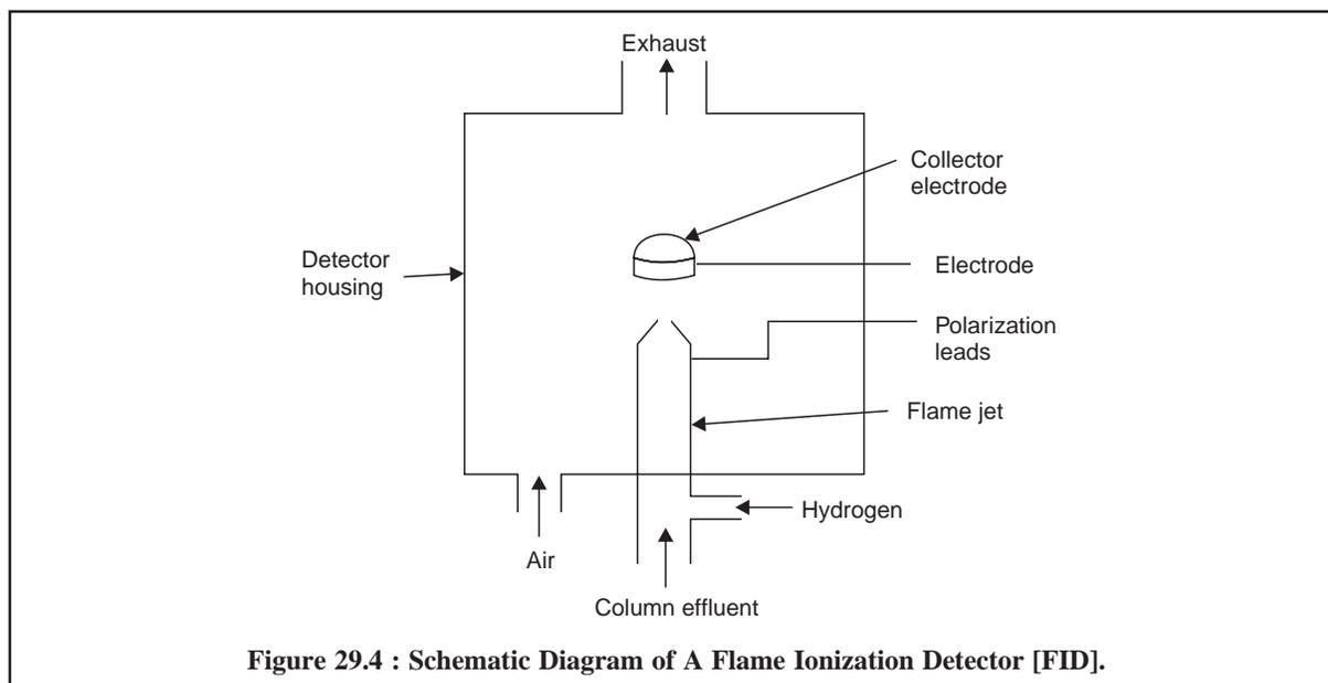
Figure 29.4 : Schematic Diagram of A Flame Ionization Detector [FID].
