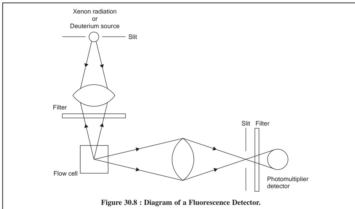
**Figure 30.8 : Diagram of a Fluorescence Detector.**
