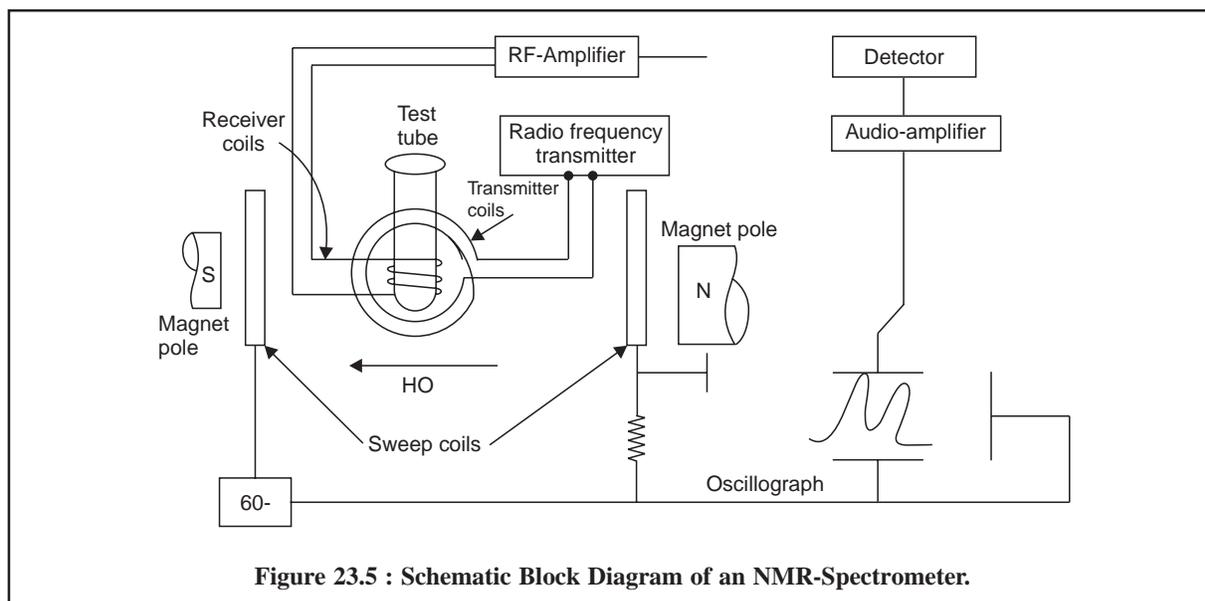
Figure 23.5 : Schematic Block Diagram of an NMR-Spectrometer.
