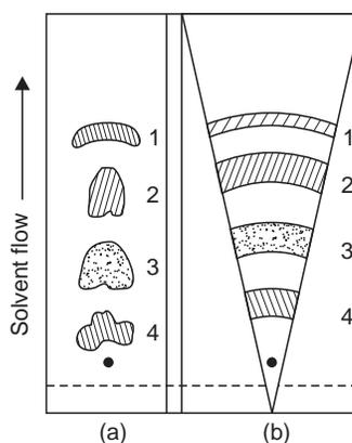
**Figure 28.5 (a) TLC-Normal technique**
