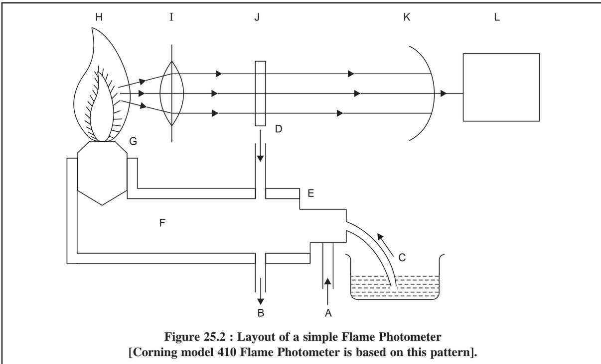
**Figure 25.2 : Layout of a simple Flame Photometer**
