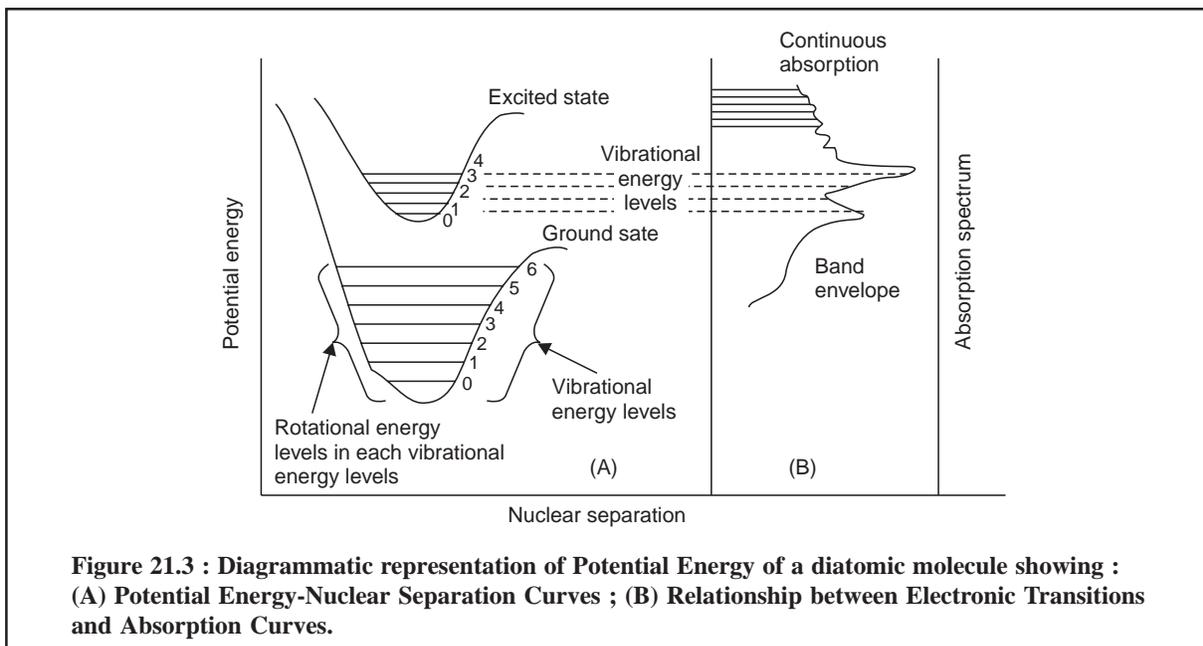
**Figure 21.3 : Diagrammatic representation of Potential Energy of a diatomic molecule showing : (A) Potential Energy-Nuclear Separation Curves ; (B) Relationship between Electronic Transitions and Absorption Curves.**
