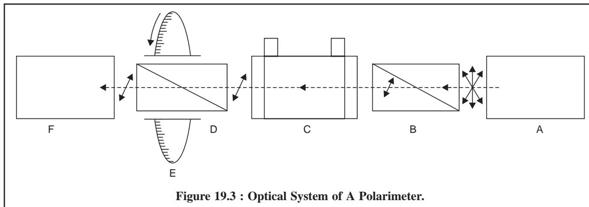
Figure 19.3 : Optical System of A Polarimeter.
