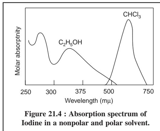
**Figure 21.4 : Absorption spectrum of Iodine in a nonpolar and polar solvent.**
