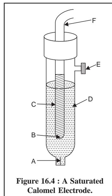
Figure 16.4 : A Saturated Calomel Electrode.
