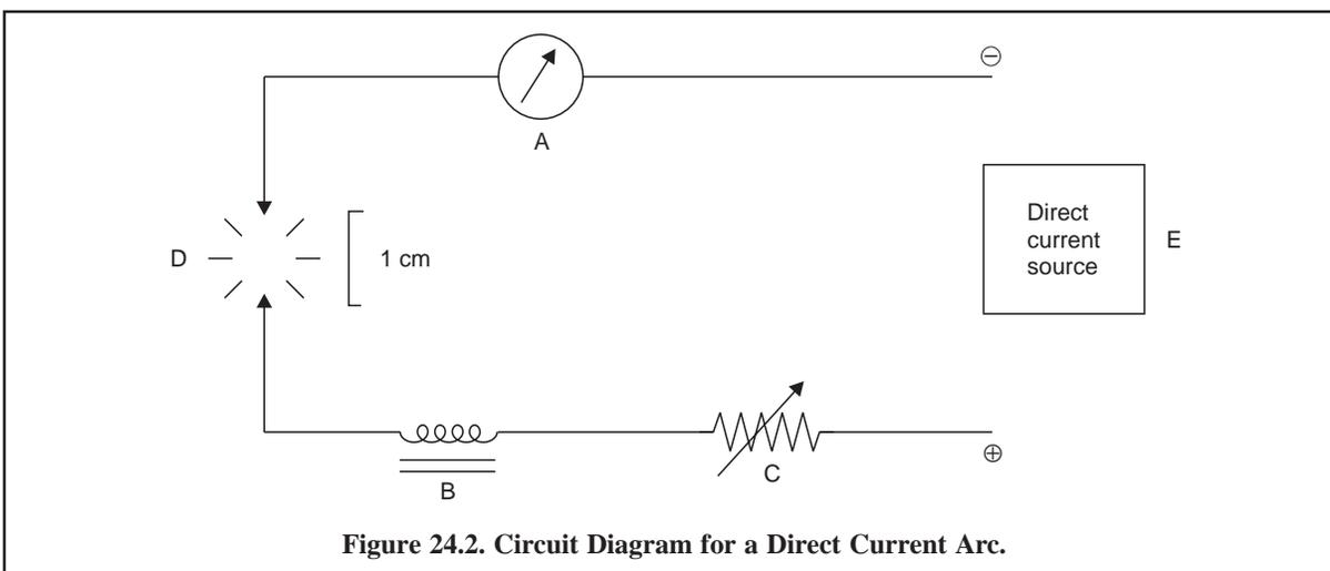
**Figure 24.2. Circuit Diagram for a Direct Current Arc.**
