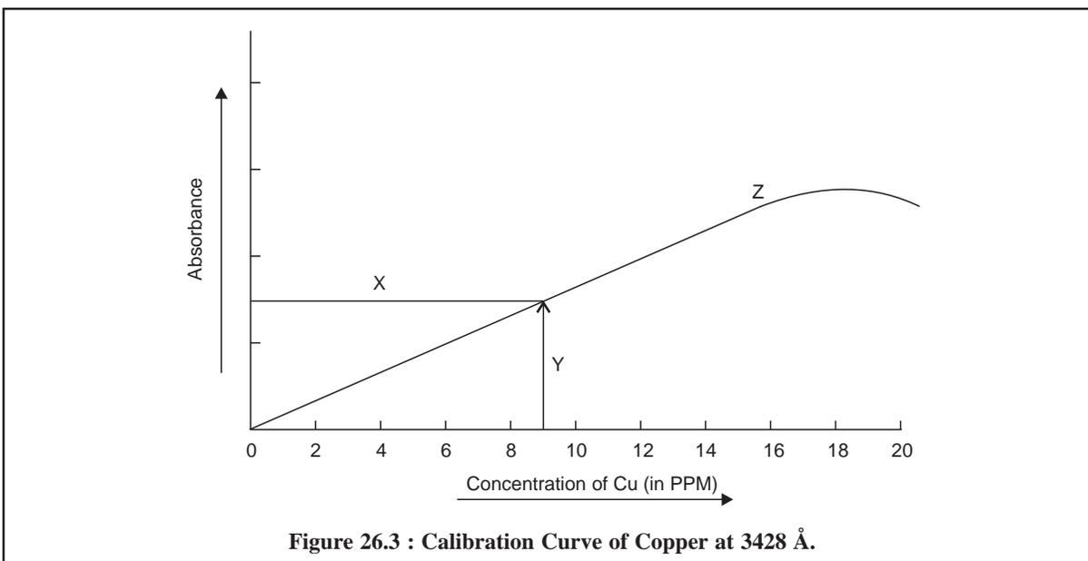
Figure 26.3 : Calibration Curve of Copper at 3428 Å.
