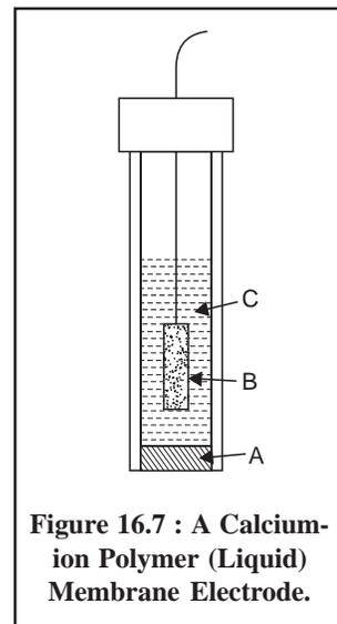
**Figure 16.7 : A Calcium-ion Polymer (Liquid) Membrane Electrode.**
