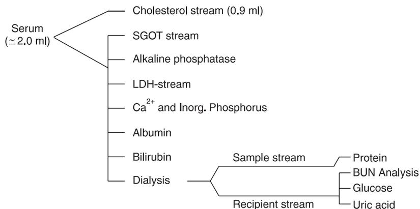
Figure 2.7 : Sample Streams of SMA-12 Survey Auto Analyzer.
