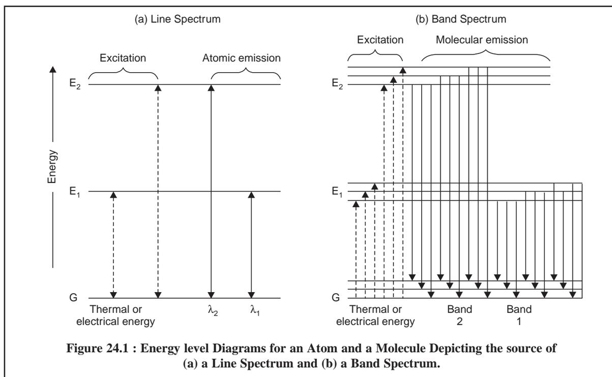
Figure 24.1 (a), designates the energy level diagram displaying the source of the lines in a typical spectrum of an element, where :
