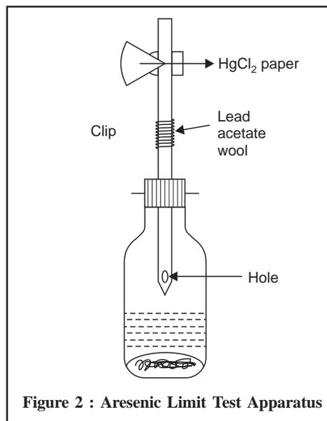
Figure 2 : Aresenic Limit Test Apparatus
