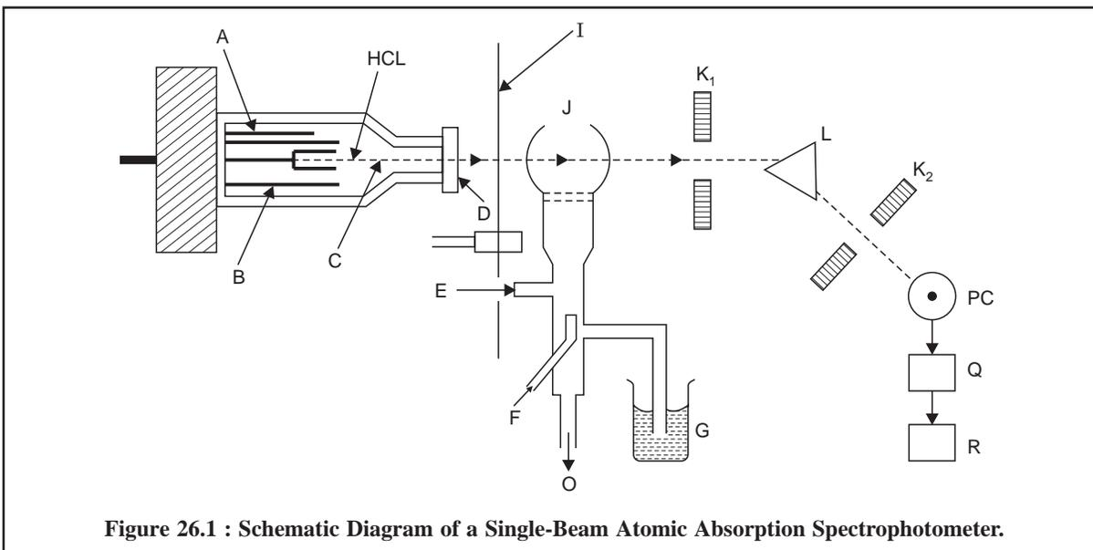
**Figure 26.1 : Schematic Diagram of a Single-Beam Atomic Absorption Spectrophotometer.**
