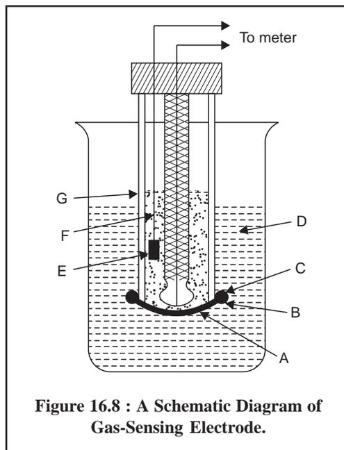
**Figure 16.8 : A Schematic Diagram of Gas-Sensing Electrode.**
