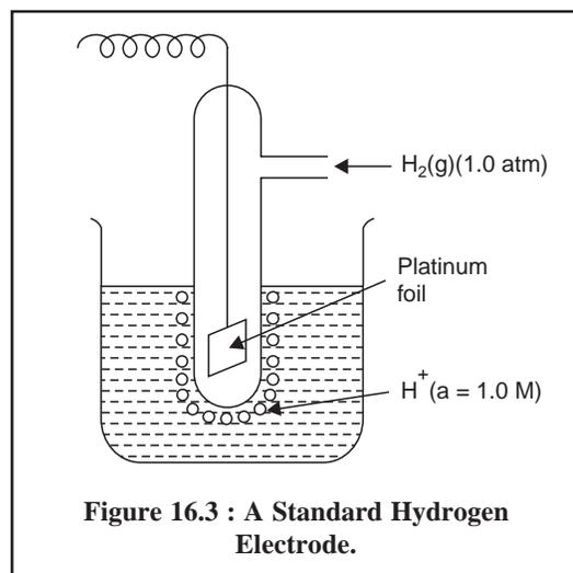
Figure 16.3 : A Standard Hydrogen Electrode.
