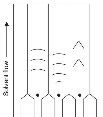
**Figure 28.4 : TLC with Wedged-Tip Divisions**
