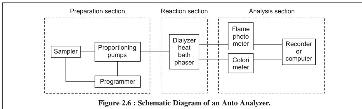
**Figure 2.6 : Schematic Diagram of an Auto Analyzer.**
