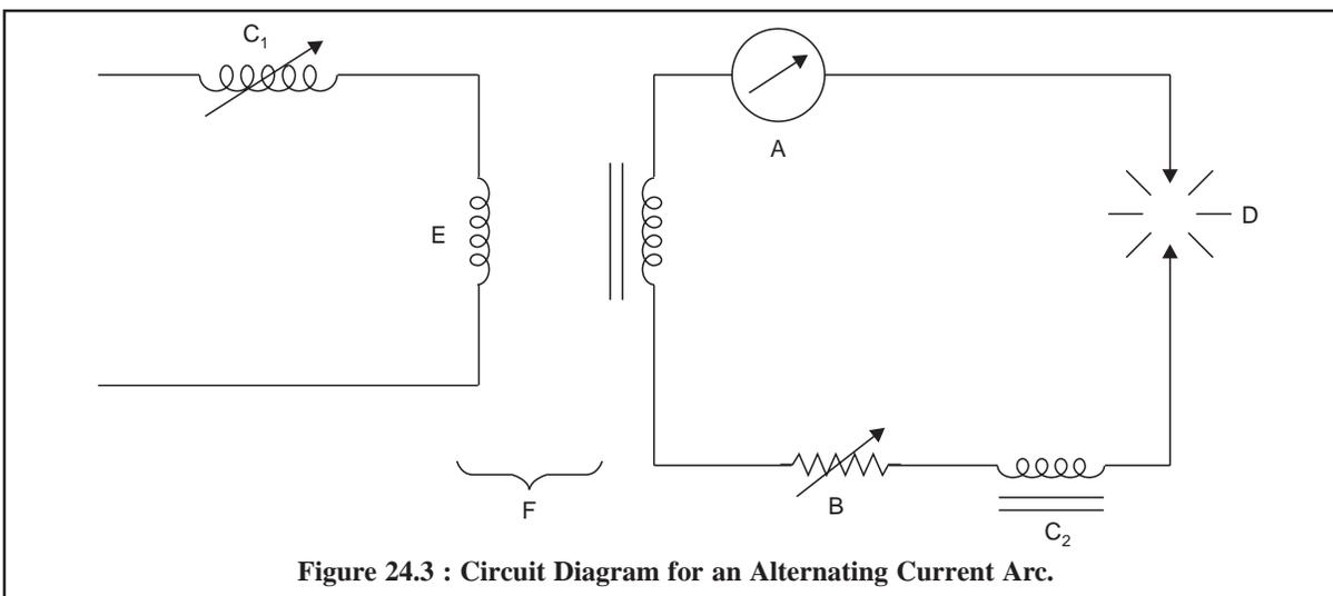
Figure 24.3 : Circuit Diagram for an Alternating Current Arc.
