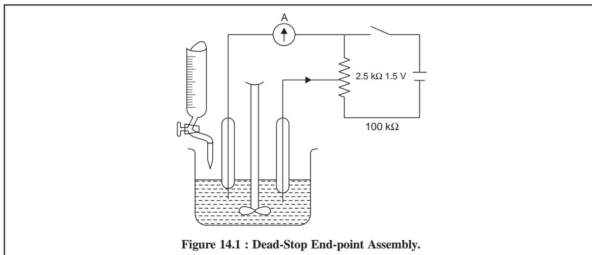
Figure 14.1 : Dead-Stop End-point Assembly.
