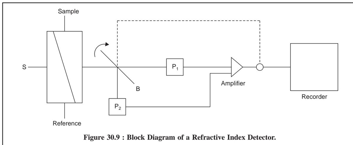
**Figure 30.9 : Block Diagram of a Refractive Index Detector.**
