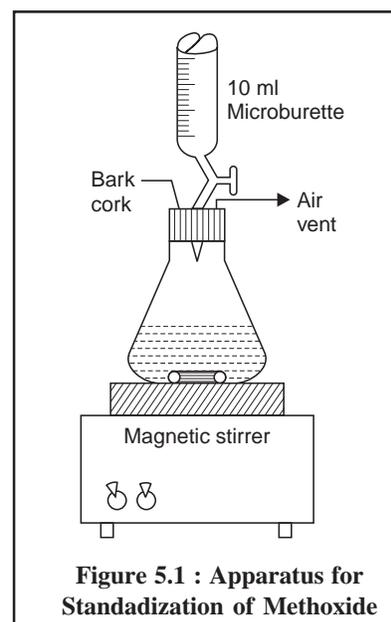
**Figure 5.1 : Apparatus for Standardization of Methoxide**
