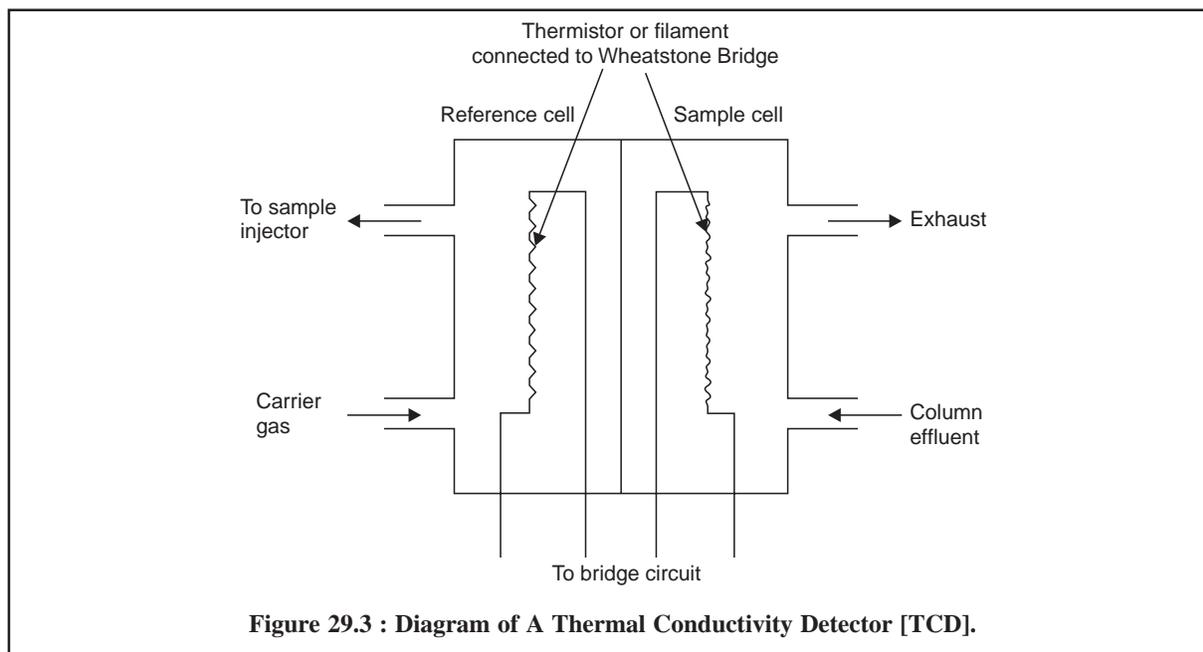
Figure 29.3 : Diagram of A Thermal Conductivity Detector [TCD].
