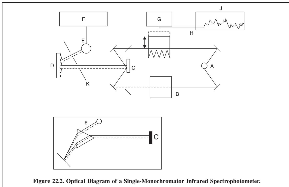
**Figure 22.2. Optical Diagram of a Single-Monochromator Infrared Spectrophotometer.**
