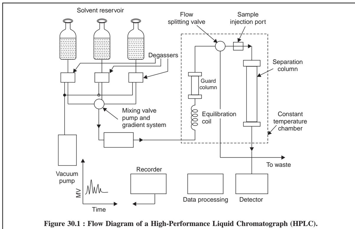
**Figure 30.1 : Flow Diagram of a High-Performance Liquid Chromatograph (HPLC).**
