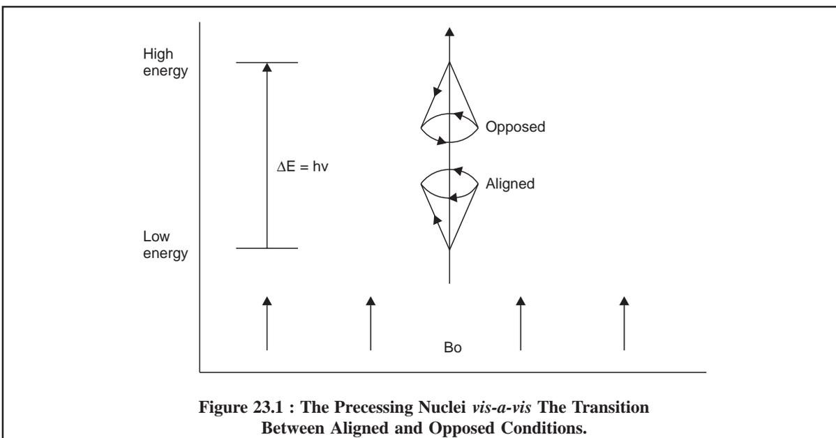
**Figure 23.1 : The Precessing Nuclei *vis-a-vis* The Transition Between Aligned and Opposed Conditions.**
