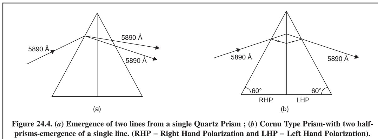
**Figure 24.4. (a) Emergence of two lines from a single Quartz Prism ; (b) Cornu Type Prism-with two half-prisms-emergence of a single line. (RHP = Right Hand Polarization and LHP = Left Hand Polarization).**
