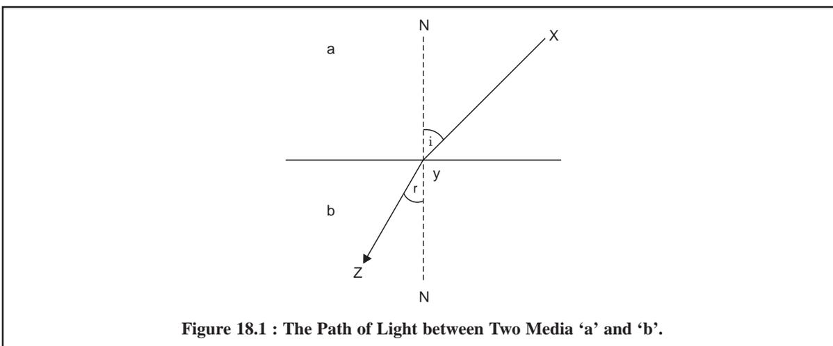
Figure 18.1 : The Path of Light between Two Media 'a' and 'b'.
