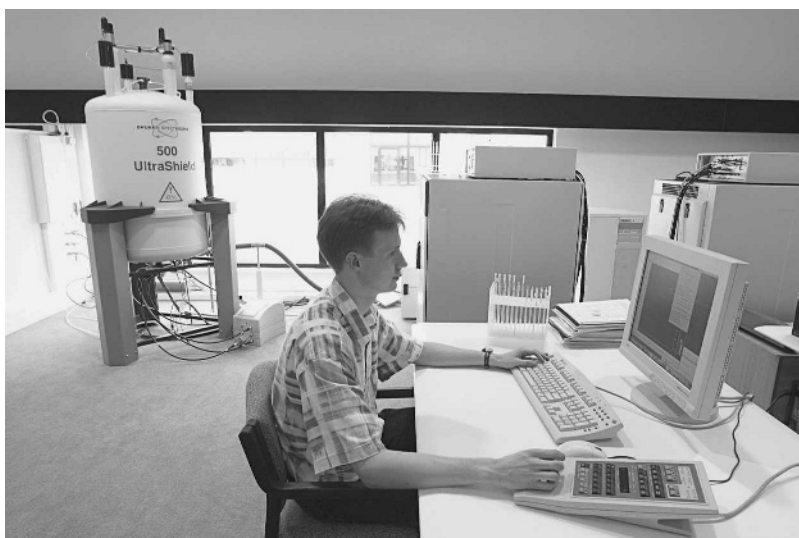
Figure 15.33 NMR research instrument. The typical appearance of these instruments corresponds, as here, to the combination of a superconducting magnet (at the bottom), of an electronic cabinet and a workstation for the analysis of results. Model Avance 400 (reproduced courtesy of Bruker).
