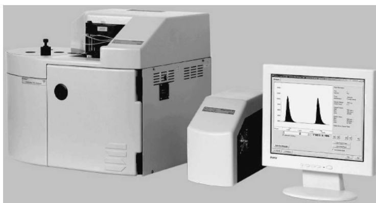
Figure 18.5 A total nitrogen analyser – model TKN, reproduced courtesy of Skalar. Detection by chemifluorescence. The small amount of light is quantified and is proportional to the nitrogen content of the sample. This type of instrument can be used for measuring proteins.
