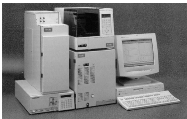
Figure 6.4 A commercial SFC installation. The oven where the column is located also controls the mobile phase pre-heating. The pump is cooled to 0°C (reproduced courtesy of Berger)
