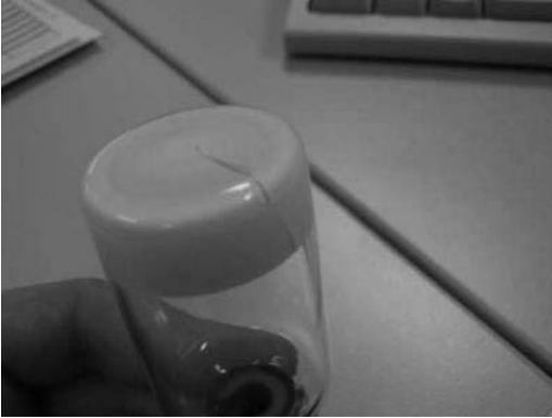
Figure 10 During a manual inspection, a crack along the bottom and side of a vial containing lyophilized product was detected.
