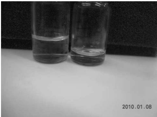
Figure 15 The vial on the right failed inspection due to less than acceptable fill volume (properly filled vial shown on the left).
