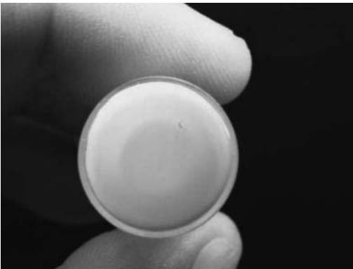
Figure 12 During manual inspection, a dark particle on a lyophilized cake is observed through the bottom of the vial.
