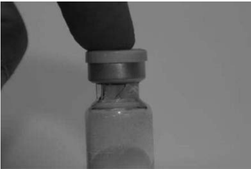
Figure 11 During a manual inspection a broken vial neck was observed.
