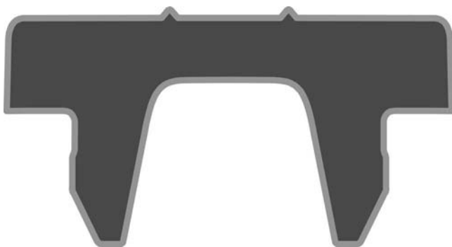
Figure 7 Totally coated stopper.
