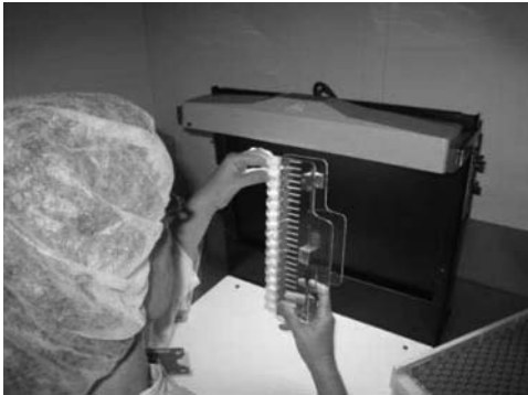
Figure 5 An inspector is monitoring vials. Here vials are placed in a clear holder so more than one unit can be inspected at a time.
