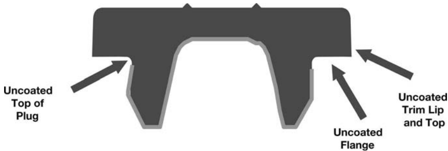
Figure 5 Plug coated stopper.
