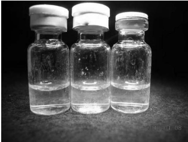
Figure 14 Photo showing vials that failed due to crimp defects, on the vial farthest right, no crimp/overseal was applied.
