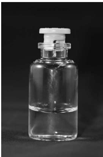
Figure 1 Freeze-dried products use a special stopper with a slot that is open when the stopper is in the partially seated position to allow escape of water vapor. The stack of shelves in the freeze dryer is compressed at the end of the cycle to force the stopper into its fully seated position.
