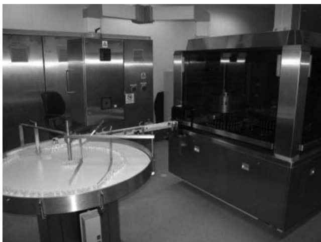
Figure 6 A photo showing the Eisai system showing vials being fed to the instrument.
