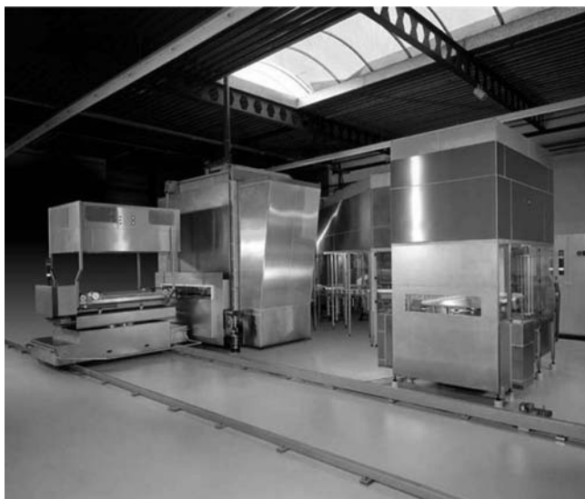
Figure 11 Lyophilizer transfer cart with loader and unloader (13).
