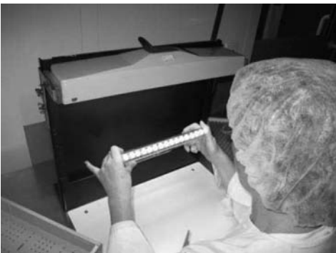
Figure 4 Prefilled syringes are inspected, ensuring that all dimensions of the product are monitored. Here the inspector is viewing the top of the syringe for any defects.
