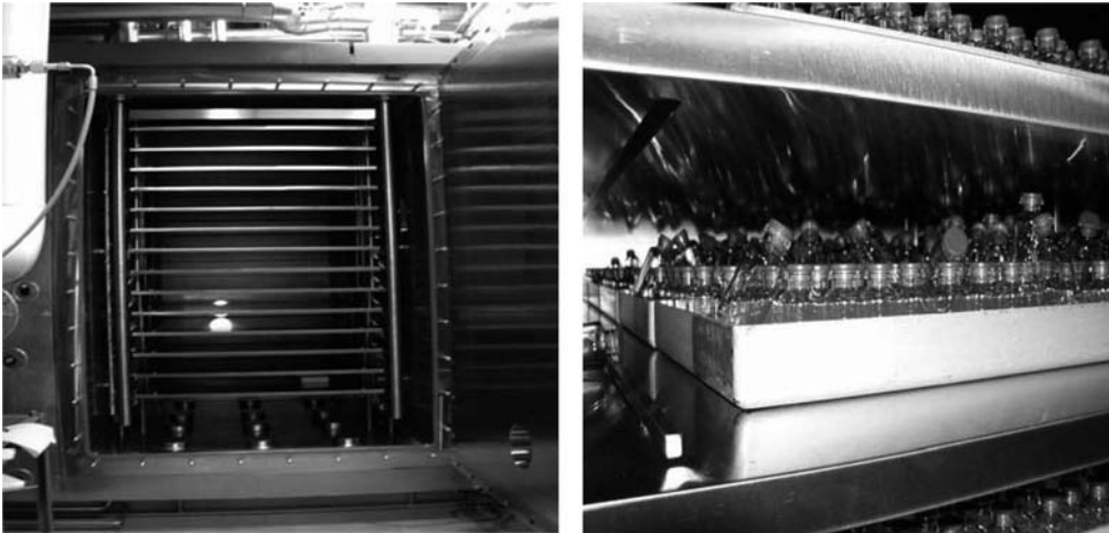
Figure 5 On the left, a picture of a pilot scale lyophilization chamber. Vials are placed on the shelves. The shelves can move so that they can bring the stoppers from their halfway down into their fully pressed down position. On the right, a picture of a shelf with vials after unsuccessful insertion of the stoppers. Stoppers got stuck to the shelf that pressed them down!
