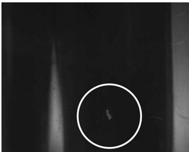
Figure 16 White particle observed in a sealed vial (circled).
