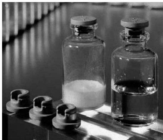
Figure 4 Lyophilization vials and their stoppers. The vial on the right hand side has a stopper in its halfway down position before freeze-drying; the vial on the left has its stopper fully pressed down after freeze-drying. In front of the vials are stoppers showing their lyophilization opening.
