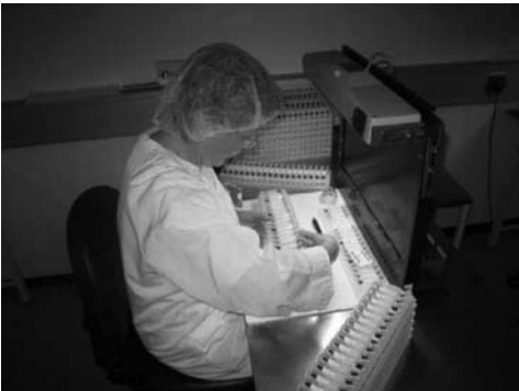
Figure 2 An inspector begins by observing the prefilled syringes in their packaging trays.
