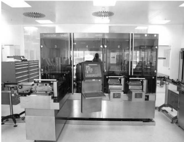
Figure 8 The Seidenader inspection machine.
