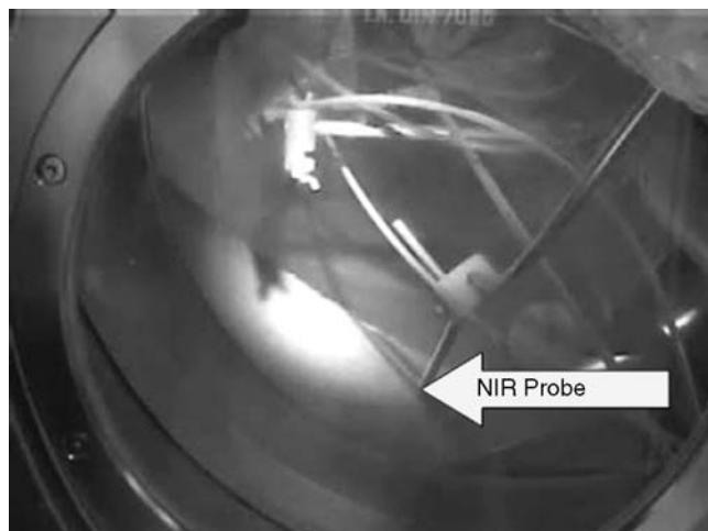
FIGURE 13 Use of near IR for pellet quality control. Source: Courtesy of Intervet. Inc.
