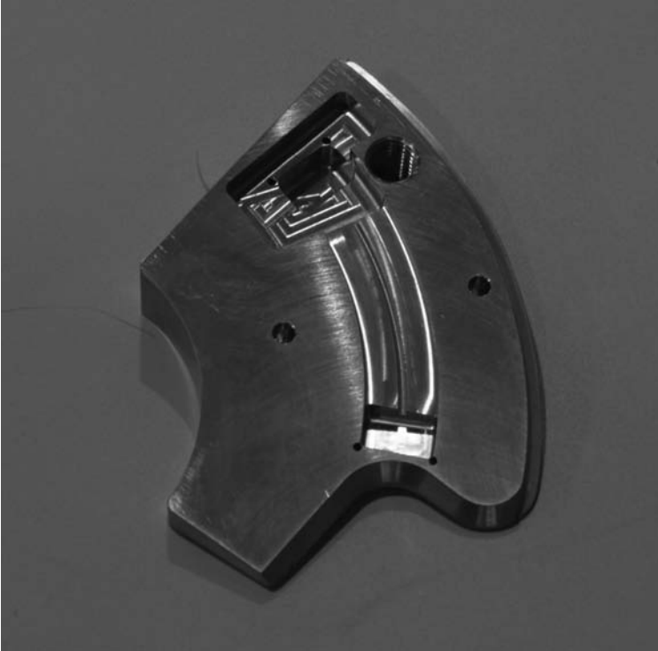
FIGURE 14 Back side of piccola ejection cam showing strain gauge pockets
