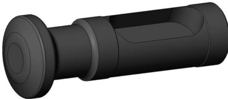
FIGURE 20 Calibrated punch pocket design.
